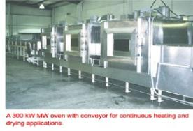
A 300 kW MW oven with conveyor for continuous heating and drying applications.
